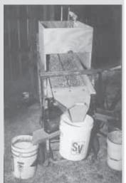
Roger Foster turned a commercial vibrating concrete machine into this portable cleaner that he uses with his corn burning stove.
