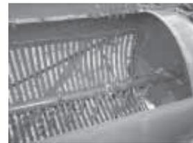
Walnuts go into one end of steel barrel and come out dehulled at other end. As chains whip around, they remove walnut hulls which fall between rerods and onto the ground. Power is provided by a 5 hp gas engine that mounts on back. Temple uses an ATV to pull shucker around his farm.
