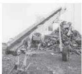
Elmer Pinkerton uses this modified chainand-paddle-type bale elevator to load firewood into big stacks.
