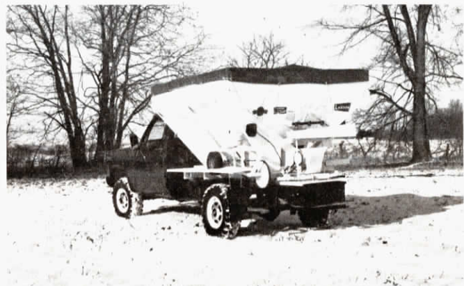
Stainless steel chain web is ground driven by a small wheel that, when engaged, rubs against one of the truck's rear wheels.
