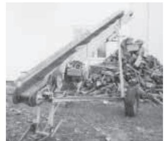
**Elmer Pinkerton uses this modified chain-and-paddle-type bale elevator to load firewood into big stacks.**
