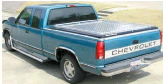
New-style pickup cover is made of high strength aluminum and will hold up to 220 lbs. Built-in rails on the sides allow you to secure the cargo.
