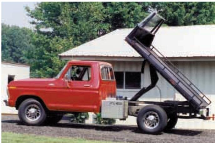
When Jerry Mattox rebuilt his 1978 Ford 3/4-ton pickup, he also equipped it with a homemade dump box and added large storage boxes on each side of the frame.
