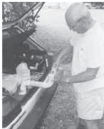
Oil from a restaurant is filtered through a cotton filter (available from restaurant supply houses). Veggie oil tank in trunk is filled via PVC gooseneck. Oil is piped to rear tank and then forward after being heated to 160 degrees.
