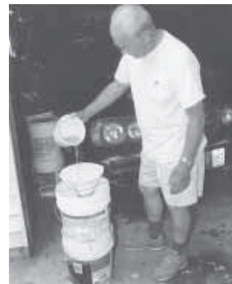
Oil from a restaurant is filtered through a cotton filter (available from restaurant supply houses). Veggie oil tank in trunk is filled via PVC gooseneck. Oil is piped to rear tank and then forward after being heated to 160 degrees.
