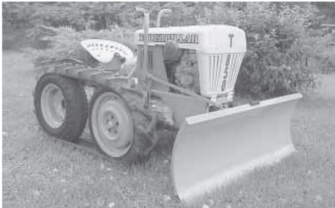
Tad Schreiner converted a Bolens garden tractor into this tracked tractor, adding an automotive rear end and tracks made from tractor tires.
