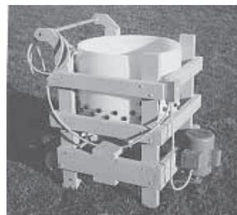
Tub-style Whizbang Chicken Plucker is housed inside a wooden frame and powered by an electric motor.
