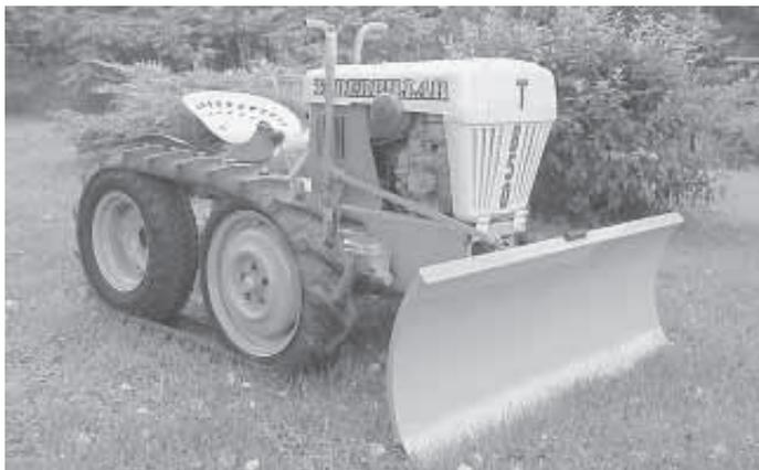
Tad Schreiner converted a Bolens garden tractor into this tracked tractor, adding an automotive rear end and tracks made from tractor tires.
