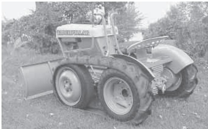
To make the tracks, Schreiner cut the sidewalls off a pair of 6 by 30 bias-ply tires.
