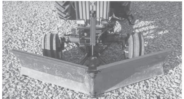
Blade raises and lowers hydraulically and also V-angles for ward or back, thanks to a hinge in the middle where it pivots on a 1 1/2-in. dia. pin.
