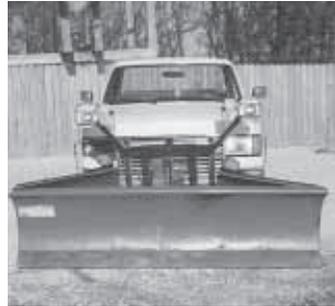
Hydraulically adjusted 3-ft. wing blades convert a standard 8 1/2-ft. snow plow into a 14-ft. wide model. For transport, the add-on blades fold up behind plow. Snow plow mounts on a Ford F-150 4-WD pickup.
