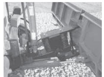
Blade can be angled up to 25 degrees from side to side via two wing cylinders.
