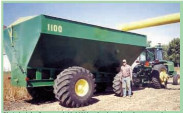
Big 4-wheeled pull-type cart holds 1,100 bu. of grain and has a front-mounted, turret-style auger that can load a semi from either side of cart.
