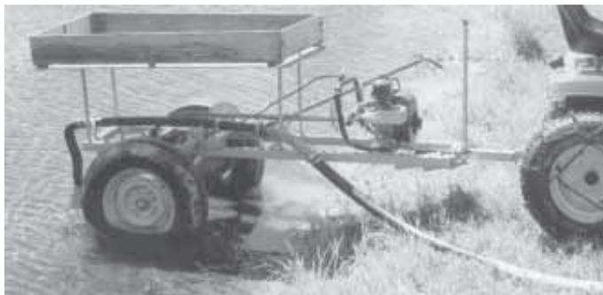
Charles Hoyt uses this trailer-mounted pump to pull water out of a nearby pond.
