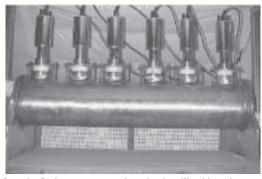
developing and testing farm-size Sonicators, as the treatment chamber is called. They've had one system in place on a 1,350-head finishing building for six months.
