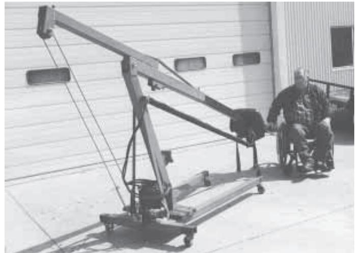
Don Skinner modified this stationary lift boom, adding a 4-ft. length of steel tubing behind the lift arm and mounting a seat on the end of machine's telescoping lift arm.
