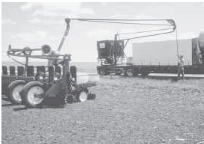
Home-built 70-ft. long "seed boom" mounts on a semi trailer and is used to fill the Sauder's 36-row, 20-in. planter. Boom hinges in middle and has 45 ft. of reach.
