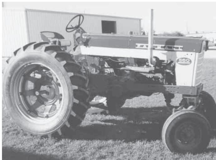
Lauer repowered this IH 560 with a 350 cu. in. V-8 engine out of a Chevrolet pickup.
