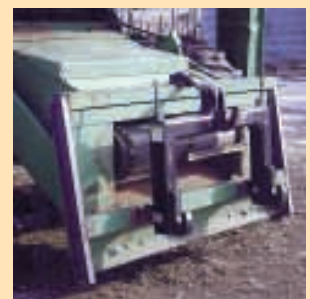
The 3-pt. header frame fits existing brackets on combine.
