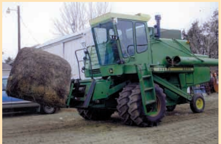
He sometimes equips the combine with a big bale fork to move bales.
