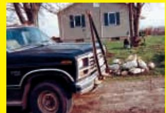
I made a towbar for my 1983 Ford F-250 pickup that mounts on the front bumper. It consists of a V-shaped metal hitch off an old rotary hoe, which bolts onto a length of angle iron that attaches to the bumper. I use the hitch to tow the pickup behind my tractor. The hitch hinges on a pair of bolts, allowing it to be folded up out of the way. (Gary Warner, 1900 N. Ave., Sheffield, Ill. 61361 ph 309 452-4293)
