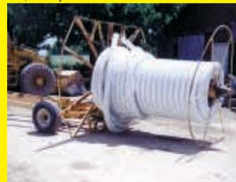
top end of the spool and then backs up and inserts the upright shaft through a 12-in. dia. pipe in the roll. In the field, a pair of hydraulic cylinders are used to tip
