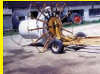
the spool horizontally to the ground. The spool can handle pipe up to 6 inches in diameter. There's 3,300 ft. of tile on a roll, and on a busy day we go through three to four rolls a day.
