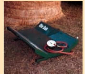
Portable cradle-type scale for round bales is 4 ft. long (left). Pickup-mounted bale spear scale is also fitted with scale (right). Operator reads weight on a 6-in. dial right behind the cab.
