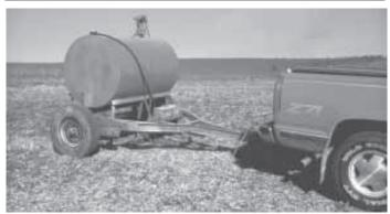
To refuel his tractor and combine in the field, Doug Eley mounted a 300-gal. fuel barrel on a two-wheeled trailer.
