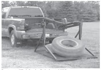
Remote-control lift platform handles loads up to 1,000 lbs.
