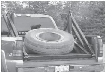
Platform stays level as it lifts load from ground into pickup bed.
