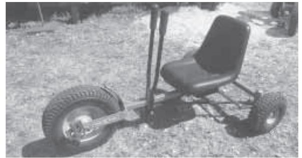
Steering on the Tig 'R Tail is controlled by a pair of levers connected by metal rods to tie rods on back.
