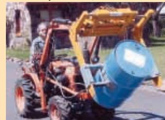
Above left photo shows unit with arms that open to a 70-in. width. Unit can also be fitted with a barrel handling attachment (right).
