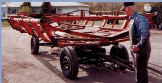
To make this feeder, Gilbert Lang removed the sickles from a couple of Versatile 18-ft. swather headers, then bolted the two heads together.
