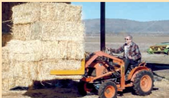
Designed specifically for utility tractors, "Mighty Mini Clamp" mounts on a front-end loader and can move large stacks of small square bales, as well as other materials.
