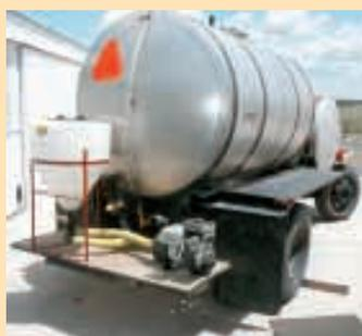
Both tanks are filled from the bottom using transfer pumps.
