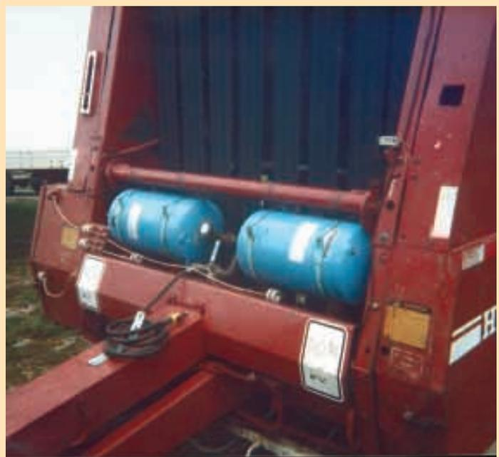
On-board fire fighting system consists of a pair of water pressure tanks, which mount in an open area above the hitch. A 10-ft. length of 3/4-in. hose is used to put out fires.
