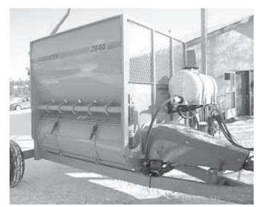
Molmixer sprays molasses liquid supplement onto shredded material as it's ejected.
