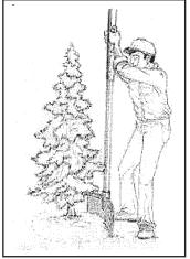
Tree spade blade is driven into ground using a ram-type driver. It cuts through roots instead of ripping them out of the ground. airway@srv.net; Website: www.airway machine.com).
