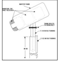
Metal water tank holds three full-size mineral or salt blocks. It sets at a 45-degree angle on a steel post that's anchored in the ground.
