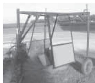
Rig's rear wheels straddle two rows of corn. A box suspended between the rows opens at the bottom for easy unloading.
