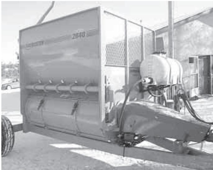
Molmixer sprays molasses liquid supplement onto shredded material as it's ejected.
