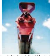
Two short lengths of auger flighting deliver grain from home-built metal hopper to twin augers. Driveshaft runs from pto shaft up to three drive sprockets.
