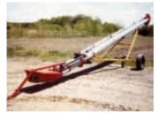
Everett Meister bought a used 60-ft. 8-in. dia. auger, cut it in half, and then put the two halves together.
