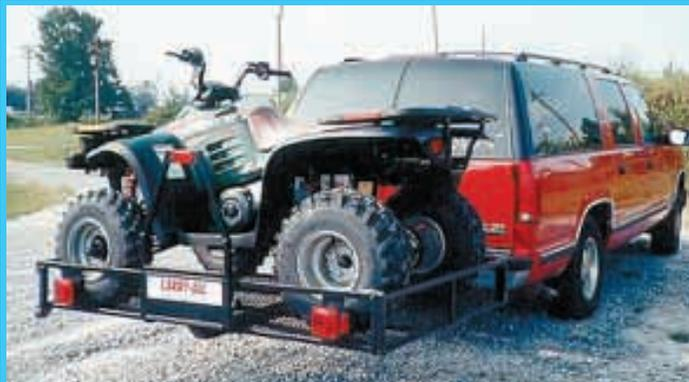
You don't need a trailer to haul your ATV. This 4 by 6-ft. rack plugs into a receiver hitch. Carries up to 600 lbs.
