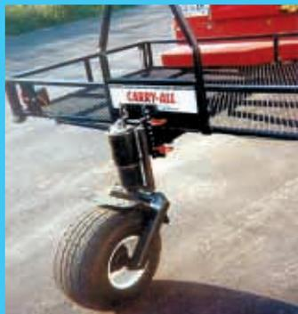
Optional support wheel on back of rack allows you to haul loads up to 1,000 lbs. jackknifing.
