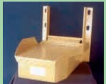
Yellow-colored steps are designed to mount on all Deere 2-cyl. row crop models back to 1935. They fit either the left or right side of tractor.
