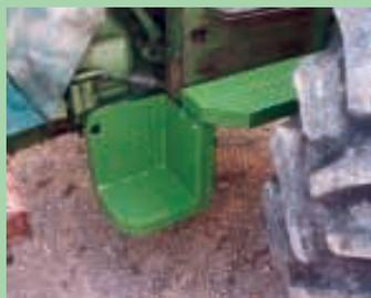
Designed for Deere 30 and 40 series tractors, these green-colored steps are built in two pieces that are hinged together.
