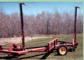
Low-profile frame holds two 9-ft. New sicklebar mowers.
