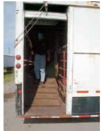
A ramp runs from lowered section of deck to main part of trailer. Rear section of trailer was lowered about 18 in.
