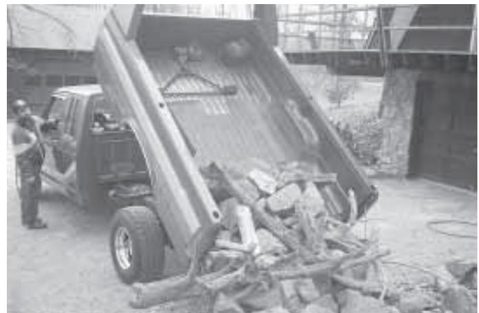
Bolt-on kit turns any full-size Chevrolet, Dodge and Ford pickup into a dump truck.
