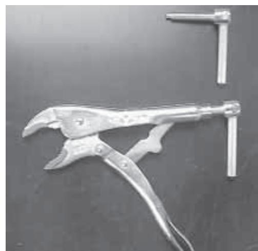
Grip-Buddy handle replaces the knob. You tighten and release the jaws with the screw-in handle, not with the spring-loaded lever.
