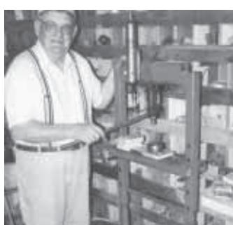
When he built this small hydraulic press, Clifford Brandenburger figured out a way to mount a 1 1/2-ton hydraulic jack upside down, resulting in a better view.
