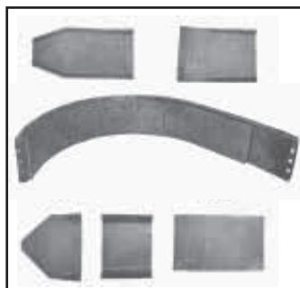
Chrome alloy liner bolts inside the blower chute. It consists of 6 1/2-in. wide overlapping sections that vary in length and shape, depending on chopper brand and model.
