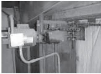
attach the motor to a 90-degree gear reduction box and speed is reduced further using a chain and sprocket to a jackshaft.
