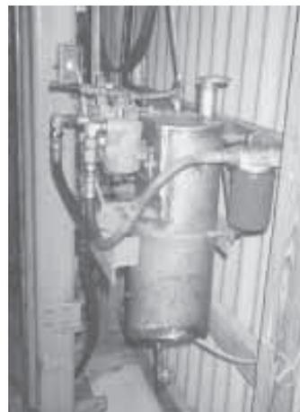
He made a power pack for the elevator from a 110-volt electric motor and a 2-speed hydraulic pump.
