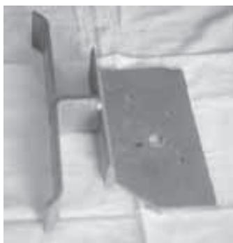
**Webster Kellogg, 4758 S. Croswell Rd., Ithaca, Mich. 48847 (ph 989 875-4221):** "When a wind storm blew a pair of big sliding doors off the track on my barn, I decided to do something about it. I made a metal bracket and bolted it to a wood plank, which I bolted to the door frame, about 8 ft. off the ground.
