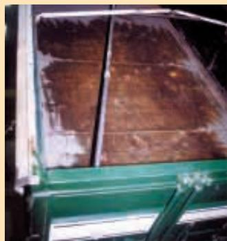
My new truck-mounted grain sampler makes it easy to collect an accurate sample from each truck load of grain. It consists of a 1 1/2-in. dia. pipe that runs diagonally about 2 ft. off the floor of the box from front to back. There are a series of 1-in. dia. holes spaced 1 ft. apart in the top part of the pipe. As grain is loaded into the truck it fills a couple inches of
