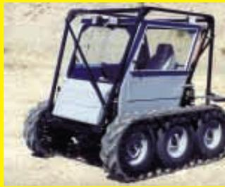
Your readers may recall the story in FARM SHOW on my home-built all terrain tracked vehicle that I call the "tank" (Vol. 25, No. 1). I built it with ordinary shop tools and low-cost, readily available components, which kept the cost way down. It rides on 11-in. wide, 8-ft. long rubber tracks made by cutting the tread out of a pair of 46-in. rear tractor tires.
