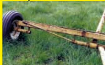
axle for it. The original axle housing was made from 2 9/16-in. inside diameter tubing with a 2 1/2-in. dia. axle bolted on inside it. I used a section of similar tubing, extending it 4 ft. on each end. The tubing is supported by 3/8 by 4-in. flat straps which I welded on above the tubing and below 20 ft. of 4-in. sq., 1/4-in. tubing. The tubing is trussed in two directions with 3/4-in. dia. rod. If I ever wanted to sell the auger I could easily convert it back to its original form.
