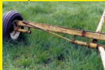
axle for it. The original axle housing was made from 2 9/16-in. inside diameter tubing with a 2 1/2-in. dia. axle bolted on inside it. I used a section of similar tubing, extending it 4 ft. on each end. The tubing is supported by 3/8 by 4-in. flat straps which I welded on above the tubing and below 20 ft. of 4-in. sq., 1/4-in. tubing. The tubing is trussed in two directions with 3/4-in. dia. rod. If I ever wanted to sell the auger I could easily convert it back to its original form.
