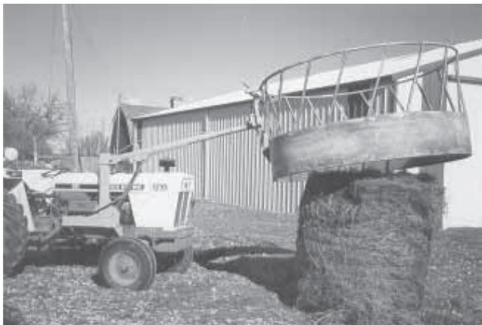
Boom consists of a single arm that’s hinged to a steel frame which bolts to tractor. “Works great for moving round bale feeders,” he says.
