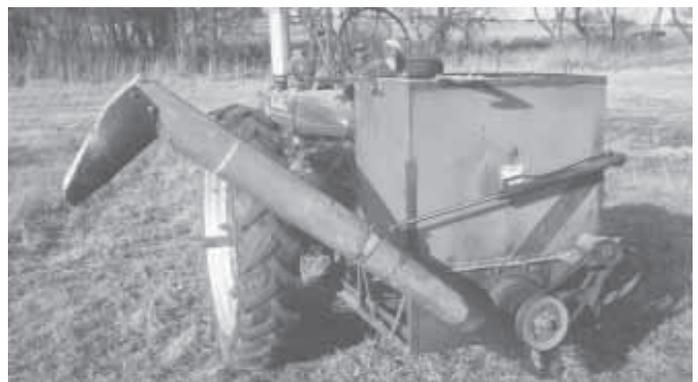
Lynn Wrosch converted the grain tank and unloading auger off an old Allis-Chalmers pull-type combine into a 3-pt. mounted, hydraulic-driven feed hopper.
