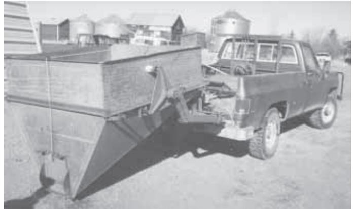
Hagg used a 1930's Case combine grain tank to make this pickup-mounted feeder. It's raised and lowered by bale-handling arms on his 3/4-ton pickup.
