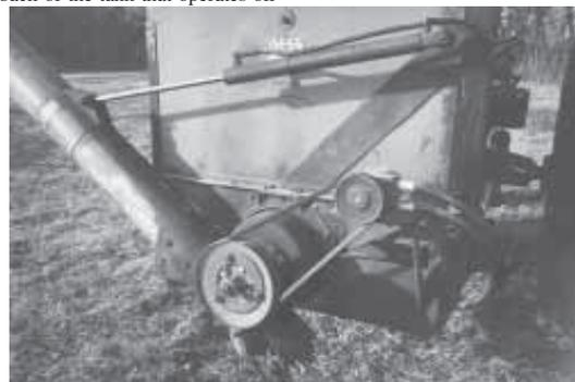
Hydraulic motor at back of tank belt-drives unload auger and auger at bottom of tank.
