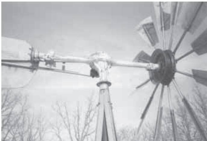
When the gearbox wore out on his windmill, McKee rebuilt it using an automotive rear end. It powers a driveshaft that runs down to a compressor at ground level.
