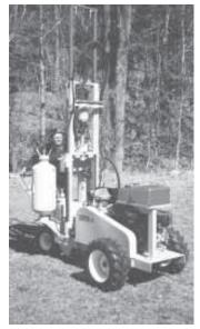
Terralift polystyrene blends into the cracks to create a network of open passage ways for liquid to drain away.
