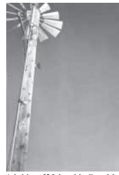
Axle drives a 35-ft. long, 1-in. dia. rod that runs to the base of pole.
