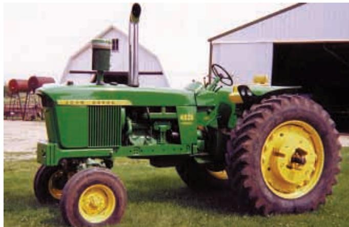
Terry Knipper repowered this 1966 Deere 4020 tractor with a used turbocharged Deere diesel engine, which came out of a 6600 Deere combine.
