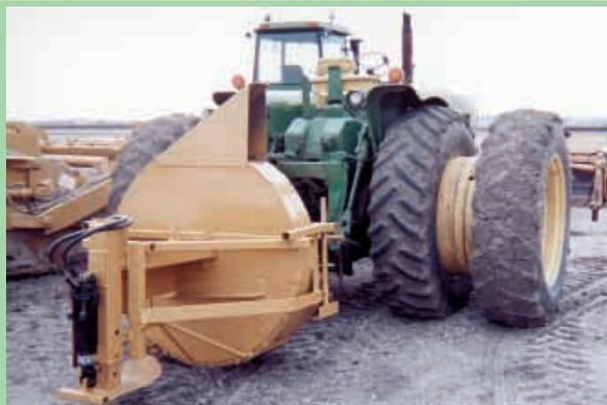
Schnack stripped a Kools silage blower down to the star wheel, pto shaft and bearings.
