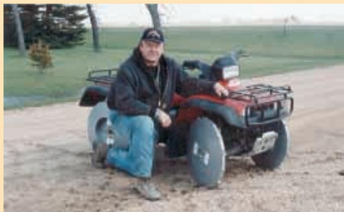
Steel "trench wheels" for ATV's are a great new way to drain excess water from fields without damaging much of the crop, says inventor Steve Raguse.
