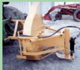
He used 1/4-in. thick steel to build a new 18-in. wide housing, leaving the bottom part open to serve as a sort of a shovel edge to cut and guide soil into blower. Homemade, hydraulic-controlled skid plate on back doubles as a depth gauge.
