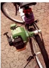
Conventional 10-speed bike was motorized with a gas engine off a Weed Eater string trimmer.
