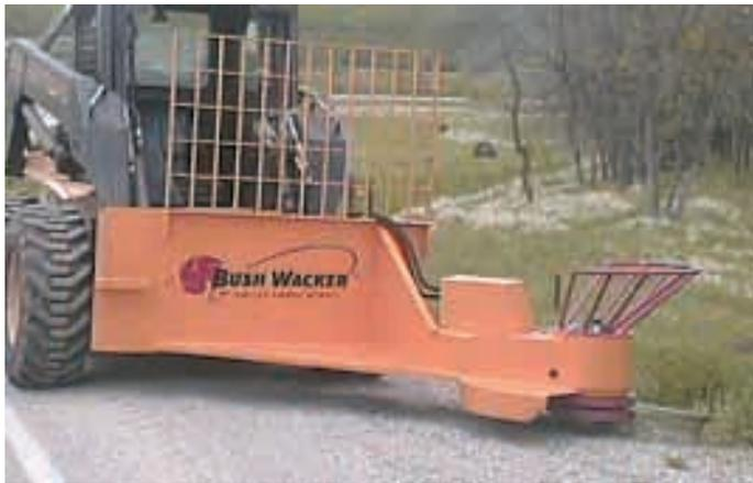
Hydraulic-powered "Bush Whacker" mounts on a tractor or skid steer loader.
