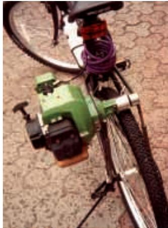
Conventional 10-speed bike was motorized with a gas engine off a Weed Eater string trimmer.
