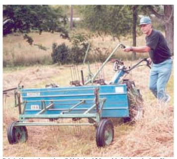
Rake/tedder attachment is available in 4 and 5-ft. models. It takes only about 30 seconds to convert rig from rake to tedder.
