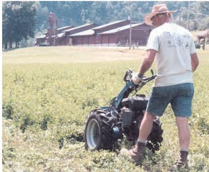
"No tractor" hay system is based on the BCS walk-behind, 2-wheel power unit. It's shown here cutting hay with a 53-in. sicklebar.
