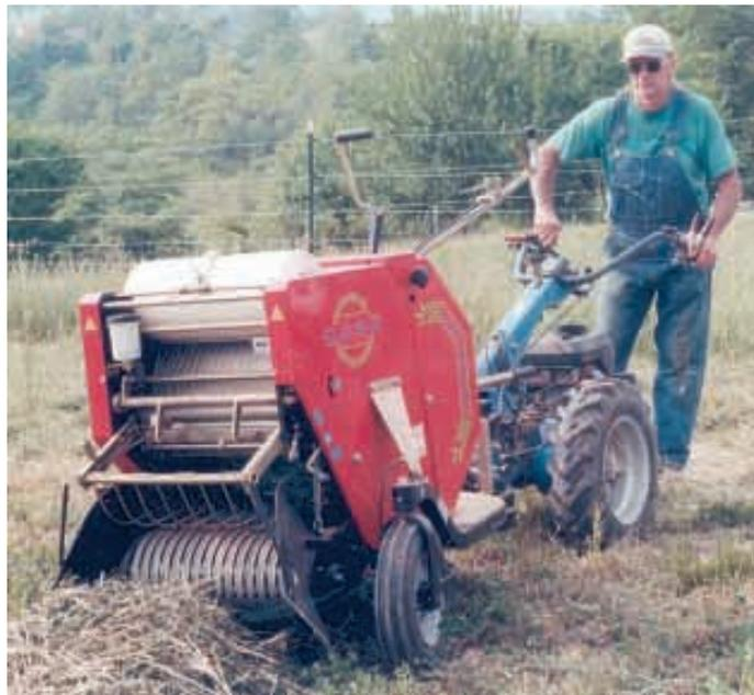
Round baler weighs 700 lbs. and produces a 23-in. bale that weighs 40 to 55 lbs.
