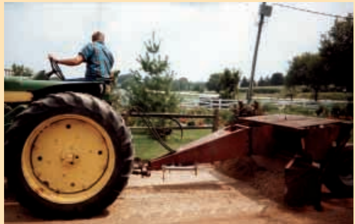
Viel cut the outside two rows off a 6-row, 30-in. planter and welded an 8-ft. snowplow blade onto the frame under the back part of hitch.
