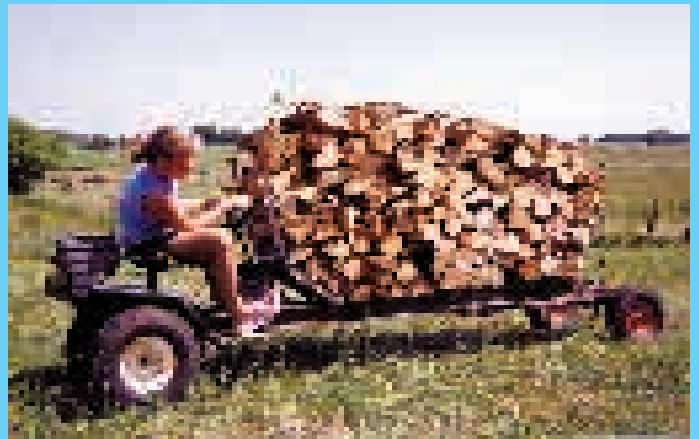
You've never seen a wood hauler like the one built by Bobby Johnson of Irvington, Ky. It's powered by the rear end out of a riding mower. Wood is carried between metal posts welded to the frame rails.
