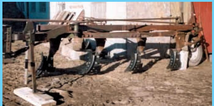
John Strockoz rebuilt an old moldboard plow, replacing moldboards with chisel shanks.
