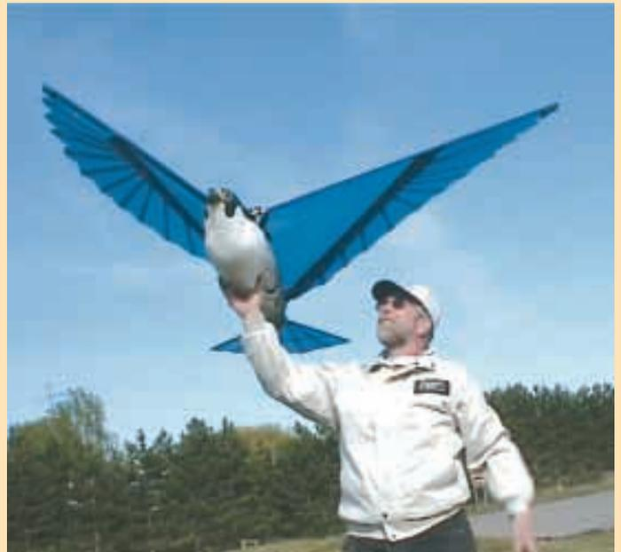
Radio-controlled "Robofalcon" soars through the sky like a hawk to scare pest birds away. It can be powered by either a gas engine or electric motor.
