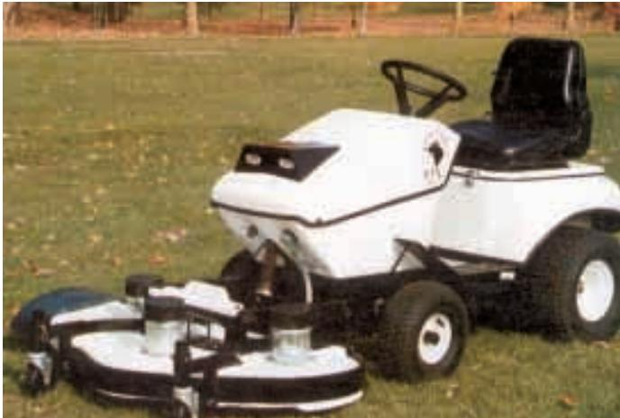
Utility tractor is powered by either a 36 or 48-volt battery pack. There's no gas or oil in the tractor, and no engine, transmission, belts or pulleys.
