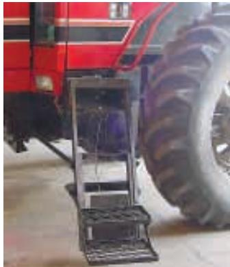
Powered by an electric winch, expanded metal steps slide up or down lengths of channel iron that bolt to tractor frame. Winch is operated by a simple up-and-down control switch that mounts on cab door.
