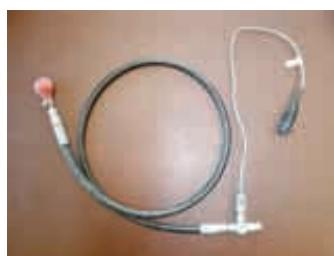
Pressure on bulb is read by either an electronic sensor or a simple dial pressure gauge.
