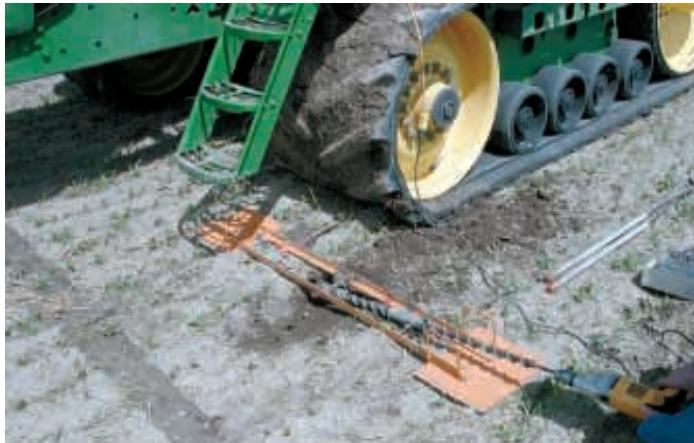
Sensor consists of a fluid-filled 1-in. dia. rubber bulb attached to a pressure transducer by a high-pressure hose. Specially-designed drill bit is used to insert bulb into soil.
