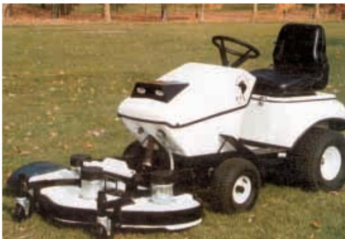
Utility tractor is powered by either a 36 or 48-volt battery pack. There's no gas or oil in the tractor, and no engine, transmission, belts or pulleys.
