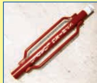
Unit has a spring-loaded plate that strikes post. After it hits, the compressed spring bounces the driver back up for the next blow.
