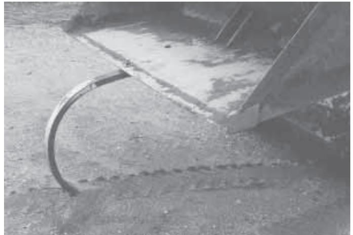
Chisel plow shank bolts onto skid loader bucket with the sweep facing backward.
